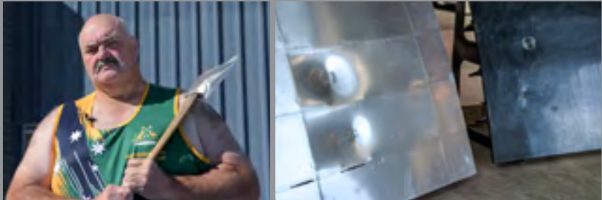
World Champion axeman, David Foster OAM took a swing at HDPE. Using similar force and the same equipment the aluminium section buckled significantly and came close to tearing. Apart from scuff marks, the HDPE was totally undamaged.
